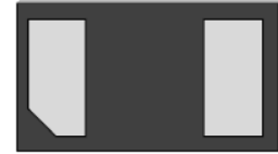
DFN0603-2L (Bottom View)
